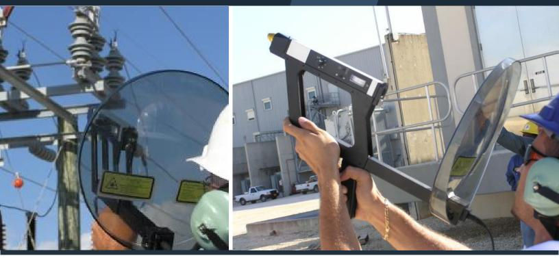
The PowerBeam 300 Was Designed To Test High Voltage Insulators And Transformers From A Safe Distance With A High Degree Of Accuracy.
